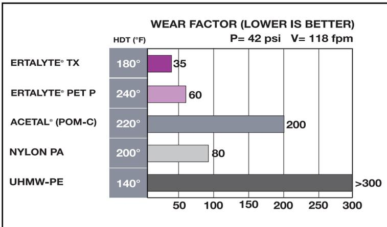
Fig. 13 - ERTALYTE® OFFERS BETTER STRENGTH IN HIGHER TEMPS
