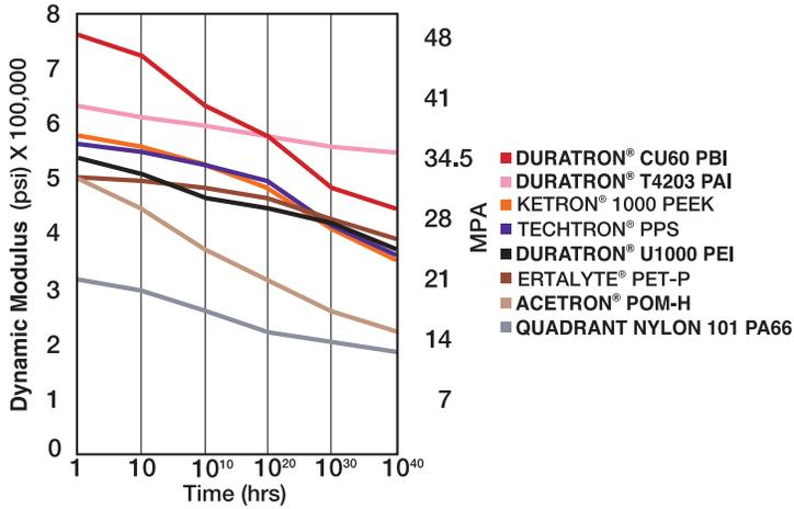
Fig.3 - CREEP AT 300°F (150°C) - DYNAMIC MODULUS - TIME CURVES
